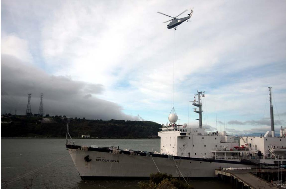
The profile of the Training Ship *Golden Bear* has been altered with the addition of a new 13-foot high, 12-foot diameter, 1,800 pound satellite antenna which will enable the ship to better communicate with the Cal Maritime campus and the world during its training voyages including live, always-on Internet connections. The new unit was lifted into place Thursday, March 13<sup>th</sup> using a helicopter.
