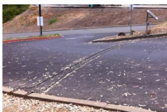
Pressure sensors and display at Lot 'E' entrance
